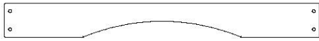
L8 | GUÍA DE PARED DE LA CASA CLUB - W100569 (x1) | 5/8" x 4 3/8" x 40" (16 x 112 x 1016)
