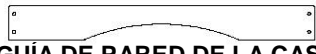
L8 | GUÍA DE PARED DE LA CASA CLUB - W100569 (x1) | 5/8" x 4 3/8" x 40" (16 x 112 x 1016)
